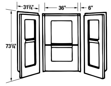
**General:** Furnish and install as shown on plans, 36" square shower, DURAWALL® Shower Walls Model 736, as manufactured by E.L. Mustee & Sons, Inc. Shall be 3-piece, molded fiberglass wall with minimum thickness of 125 mils and mounts direct-to-studwalls. Includes center panel with molded-in shelves and two side panels with molded-in shelf. Self aligning panels use a tongue-and-groove connection. Shall meet ANSI Z 124-2011.2. Color\_\_\_\_ (White, Bone).
